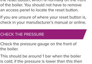
many boilers won't restart for safety reasons. You can use the filling loop to top up the system with more water to correct the problem of low pressure.
