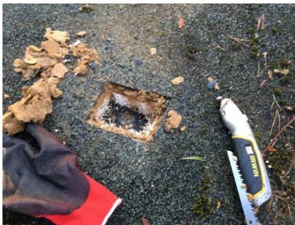
Core sample showing build up from the asphalt upwards.
